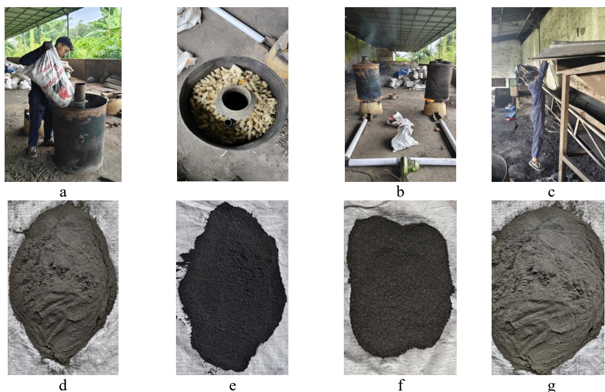
Figure 1. (a) Burning Drum, (b) Material Charcoaling Process, (c) Crusher Mill, and Fine Charcoal from (d) Cassava Stems, (e) Bamboo Stems, (f) Coconut Shells, (g) Corn Cobs
